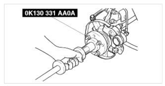
3. Remove the outer bearing, outer oil seal, outer bearing race and spacer from the wheel hub by using the SST.
