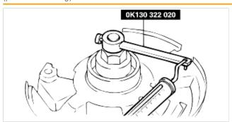
6. If the preload is not within the specification, select the proper spacer from the table to adjust it.
