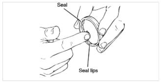
6. Install the new inner oil seal in the bore.
