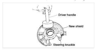
2. Install the bearing races in the steering knuckle.
