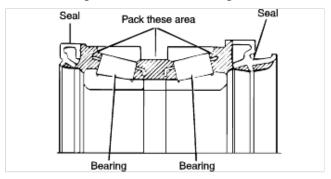
4. Place the inner bearing into the steering knuckle bore so that it rests in a level position.
