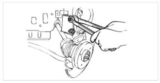
11. Separate the front hub and the knuckle from the driveshaft.
