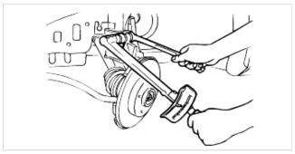
4. Install the disc rotor.
