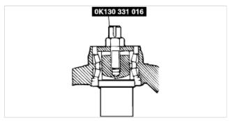
3. Tighten the nut of the SST to the specified torque.
