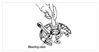
3. Pack the bearings with the Lubricant lithium grease. Pack the hub area as shown in the figure.
